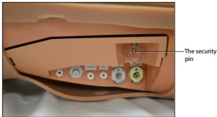
The Battery Compartment and Ports with Cover
